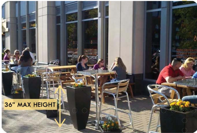
Figure 4. Max height of barriers is 36 inches.
