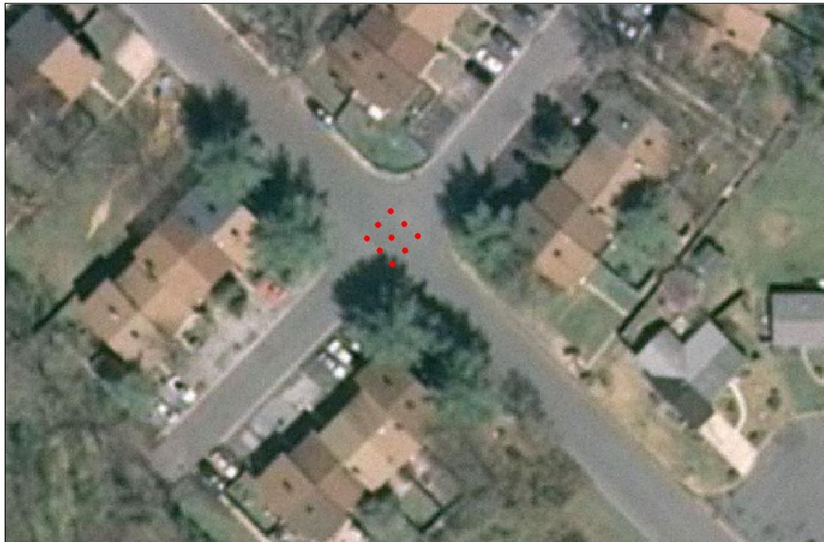
**Figure 12: 9-Point Calibration Site Example**
