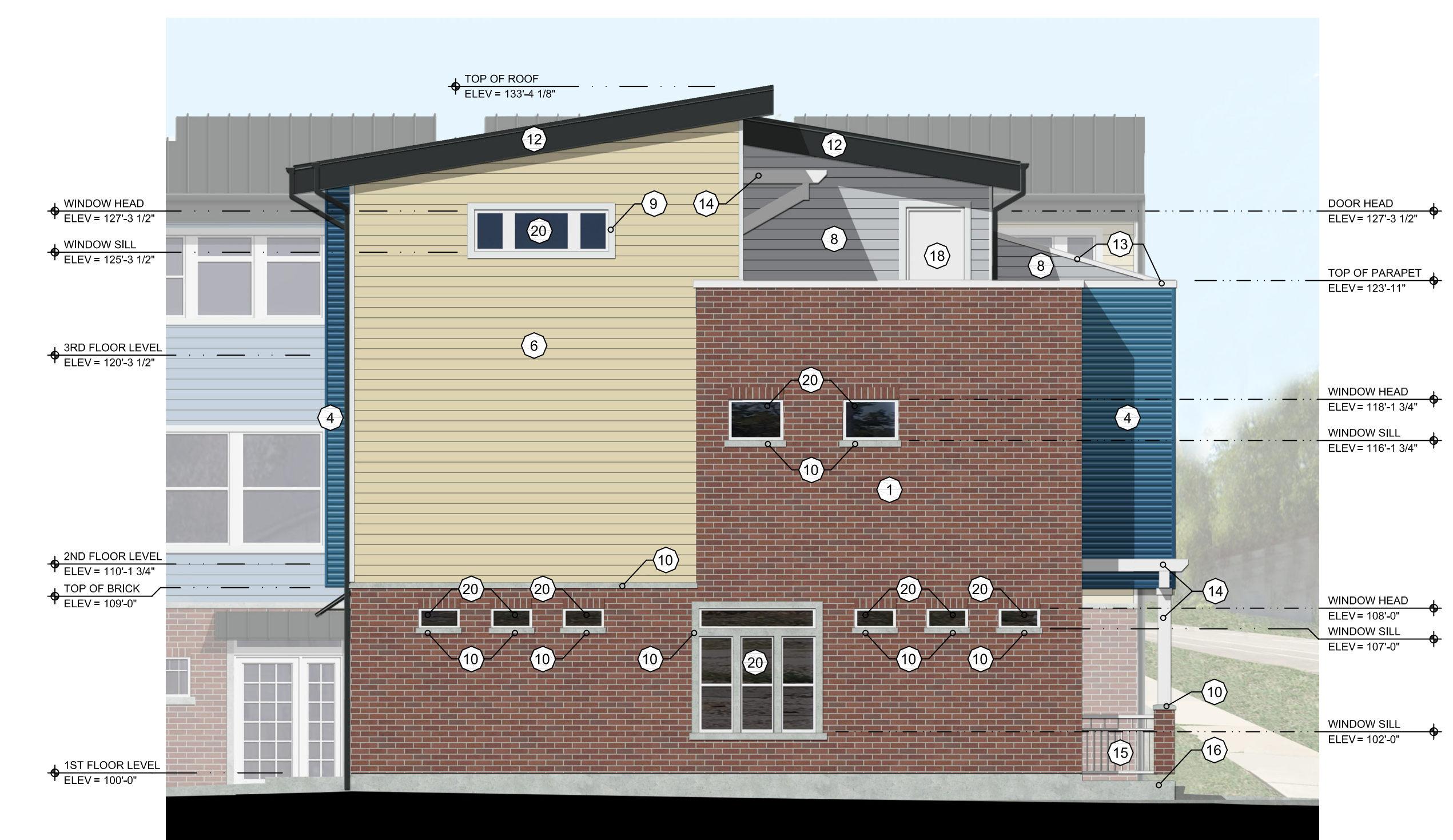
B 200 SOUTH BUILDING (WEST ELEVATION) SCALE: 3/16" = 1'-0"
