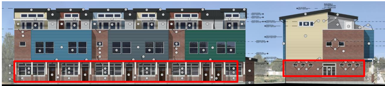
200 South and 1000 West (south façade) elevations showing the ground floor glass between 3-8 feet.
