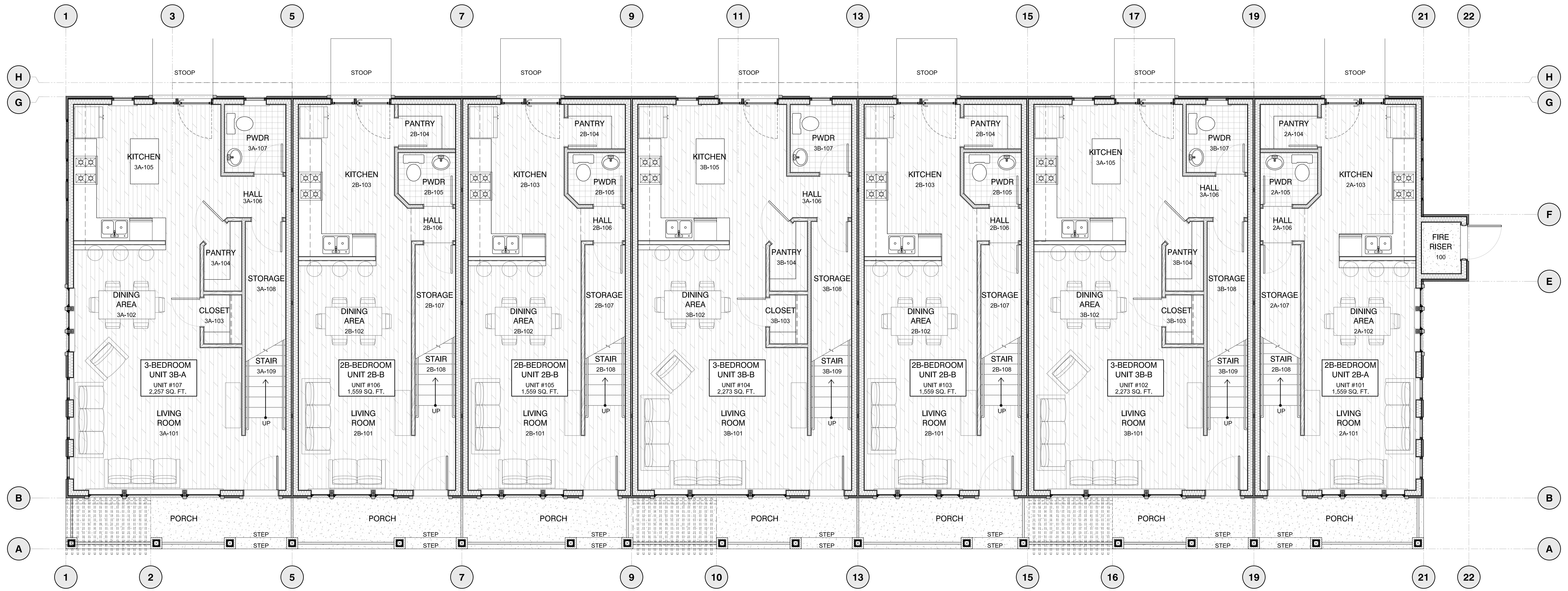
A BUILDING 1 - OVERALL MAIN LEVEL FLOOR PLAN
