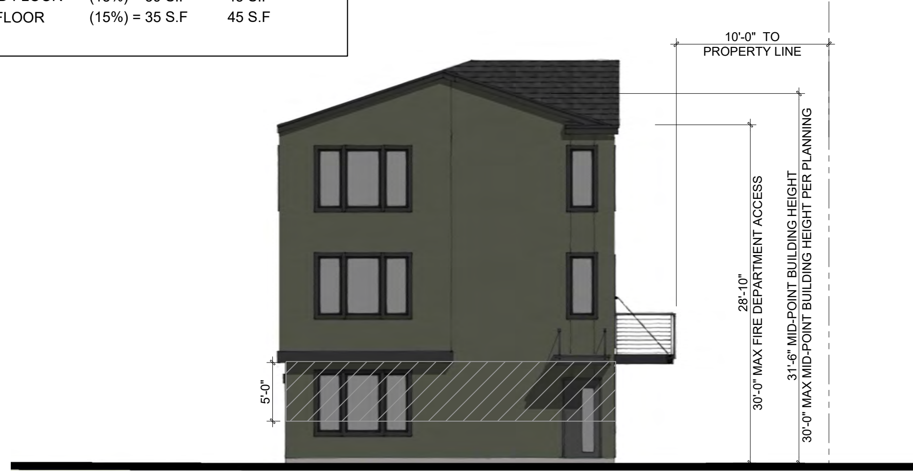
LEFT BUILDING ELEVATION - SIDE ENTRY SCALE: 1/8"=1'-0" 4
