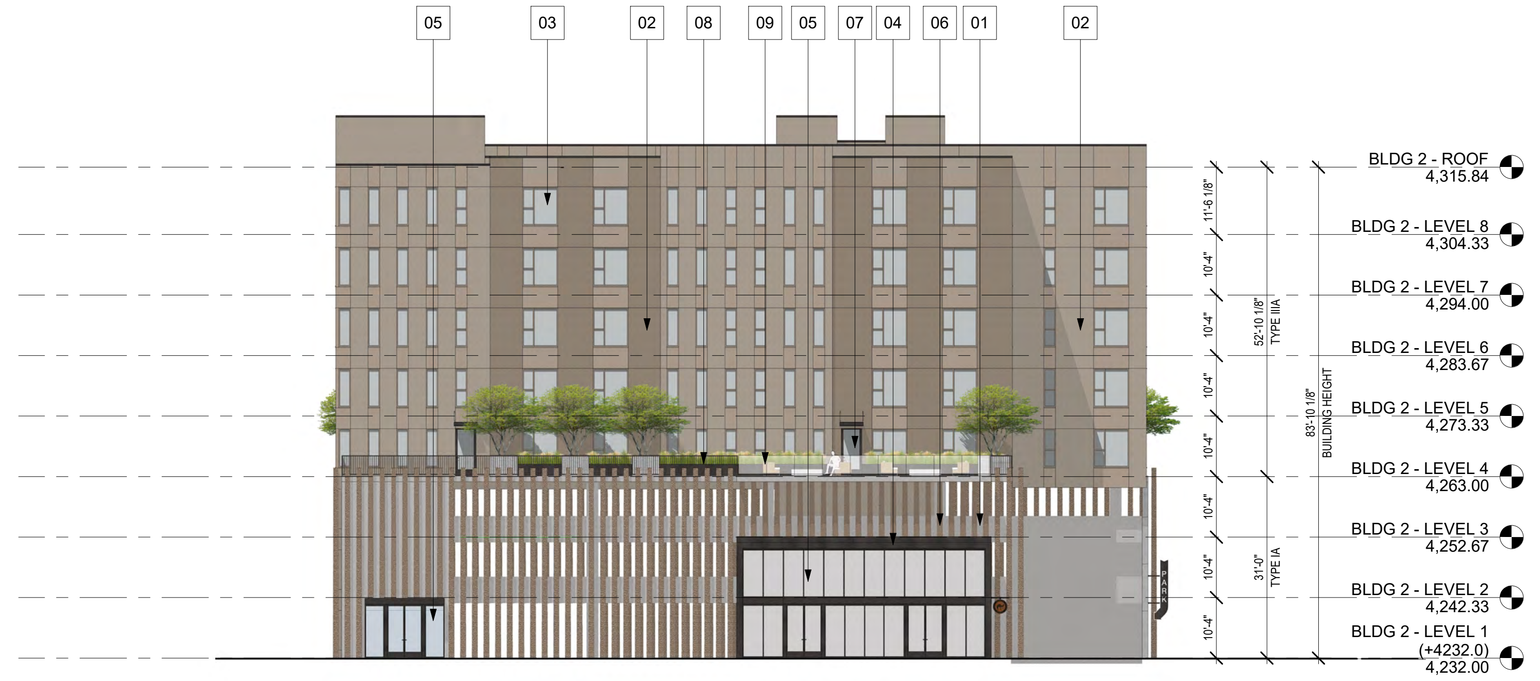
BUILDING 2 - EAST ELEVATION 1/16" = 1'-0" 2
